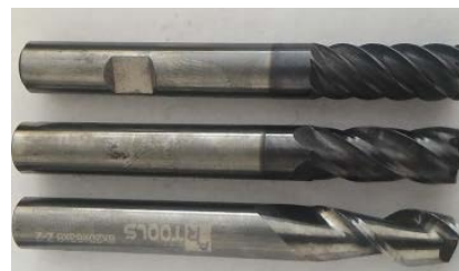
Figure 1. Vertical and inclined milling details. 2-4-6 flute End-Mill Tools Used in The Experiments
