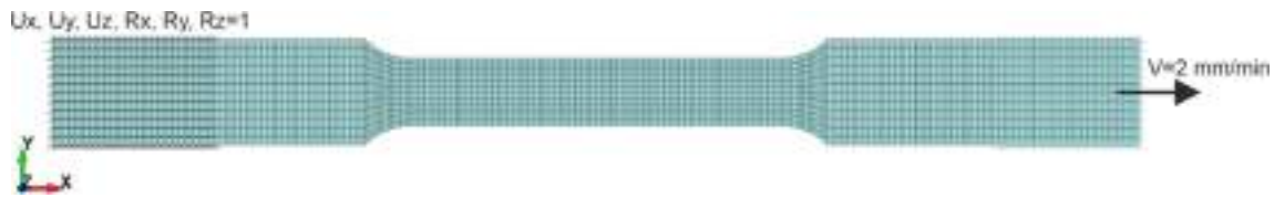
Fig. 28. Tensile test model and boundary conditions of base materials.
