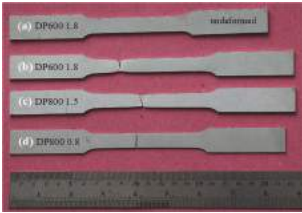
Fig. 11. Fracture images of the base materials after tensile tests.
