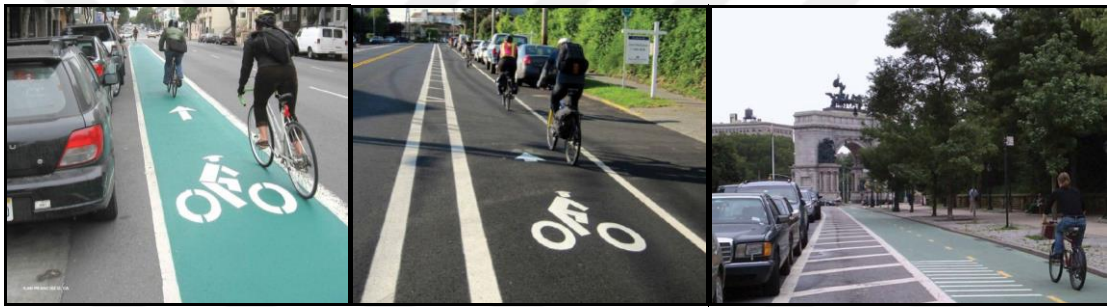
Figure 2.14 Types of cycle lanes (NACTO, 2014)
