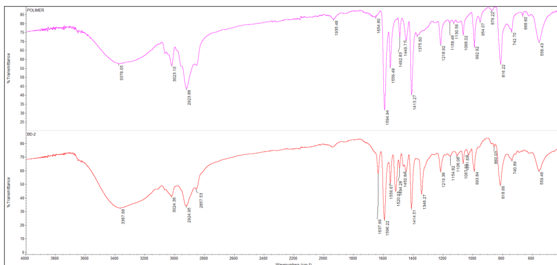
Figure 4.2. FTIR result of unfunctionalized polymer (P4VP, pink) and compound 1 (red). (n=3).
