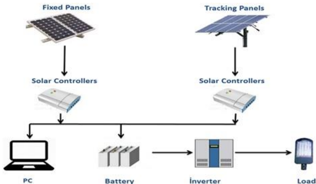
Figure 1. The block diagram of the constructed pilot solar energy production system which includes both fixed panels and dual-axis tracking panels.
