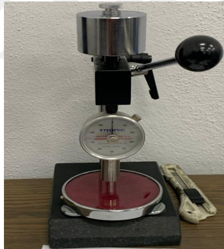
Şekil 6.5. LAC-YJ model durometre (Shore A)
