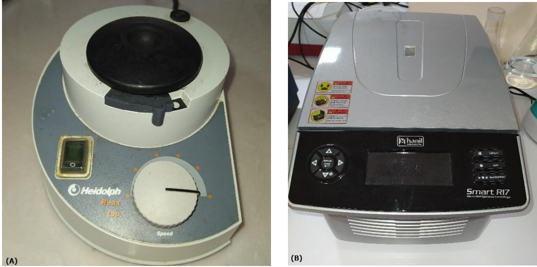
Şekil 3.4: (A) Vortex Cihazı (Heidolph®, Heidolph Instruments GmbH & CO., Schwabach, Germany); (B) Santrifüj Cihazı (Hanil® Hanil Scientific Inc., Gimpo, Korea)
