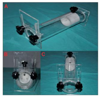
Figure 1. Transparent plexiglass cylinder apparatus for immobilization stress
